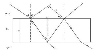
Figure 6 the optical path beams output from multiple reflections in the glass
