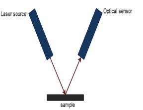
Figure 2, the trigonometric method
