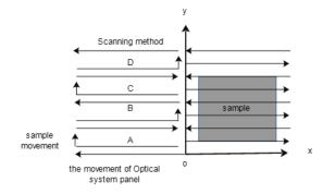
Figure 3, the laser scanning method
